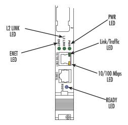
Figure 4. Model 6081RC LEDs
